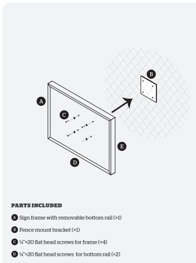
E Edge trim to to minimize fence contact with frame (×1)
