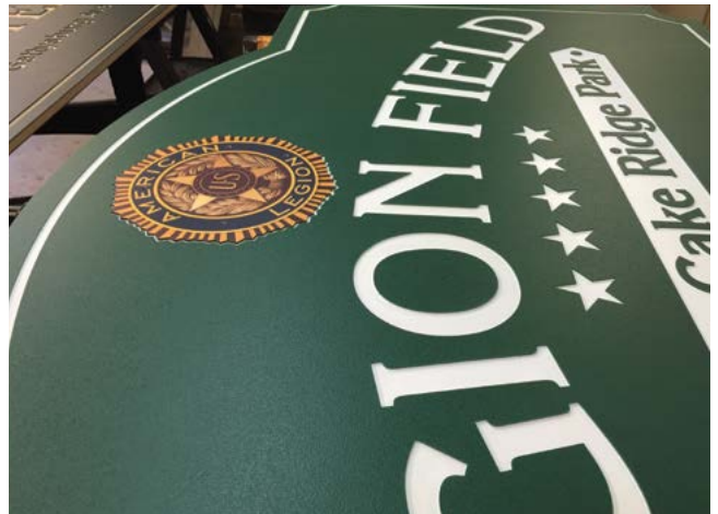
Flat routed text on green / white / green HDPE sign board with full color detailed American Legion logo achieved with TUFF COVER logo insert. A "pocket" is flat routed to accept logo.
