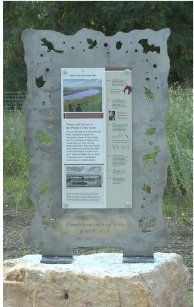
Custom cor-ten upright with laser cut icons.
