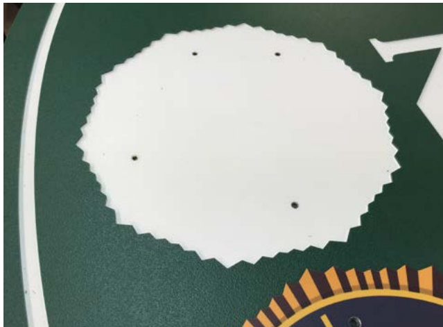
Flat routed pocket to accept logo panel insert.
